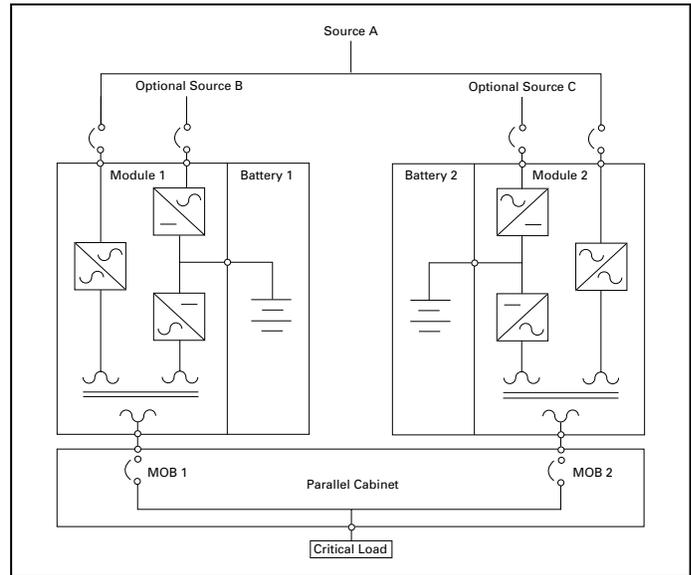
Typical 10 - 500 kVA Hot Sync Redundant Application
