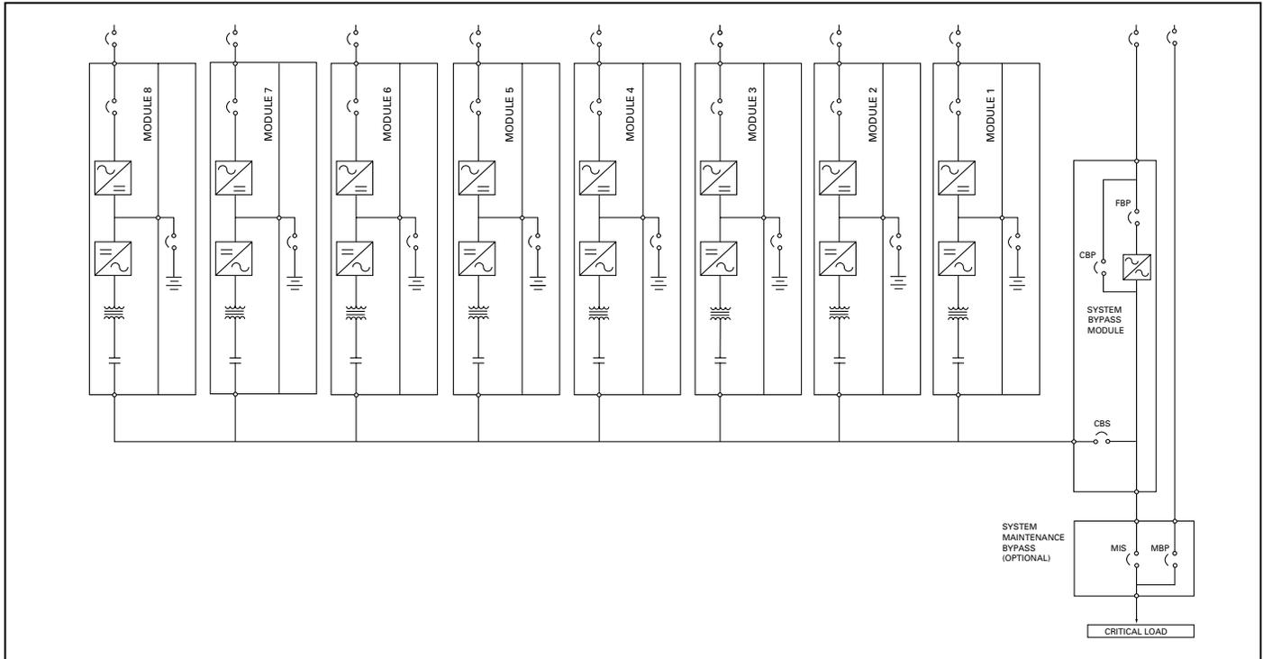
**Typical Eaton 9315 200 - 750 kVA Hot Sync Capacity Application**
